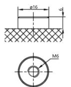
Terminal Torque Values in-Ib(Nm):17.69-26.53(2.0-3.0)
