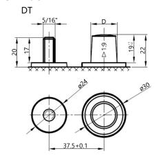
Terminal Torque Values in-Ib(Nm):17.69-26.53(2.0-3.0)
