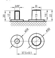
Terminal Torque Values in-Ib(Nm):17.69-26.53(2.0-3.0)
